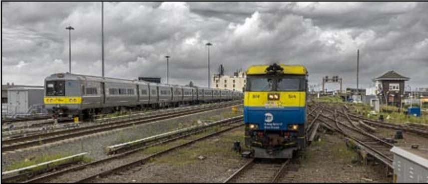
At the west end of the Long Island Railroad Station in Jamaica, New York, we see on the left, a rare M3 passenger set whose days are numbered. On the right EMD DE30AC 514, one of 24 diesel-electric only locomotives, brings in a Long Island City origin train. That is because it cannot enter Penn Station. The Long Island Railroad does have 20 Dual mode (DM30AC) locomotives that can serve Penn Station. – Two photos above © Dennis Livesey.
