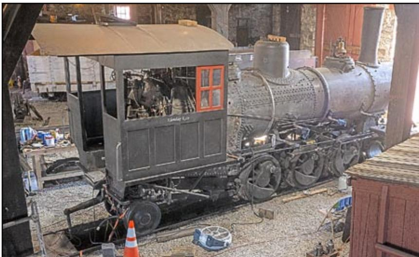
Klondike Kate #4, a Baldwin 2-6-2 built in 1912, is being converted to an oil burner at the roundhouse in Como, Colorado. – Photo © 2022 by Chip.
