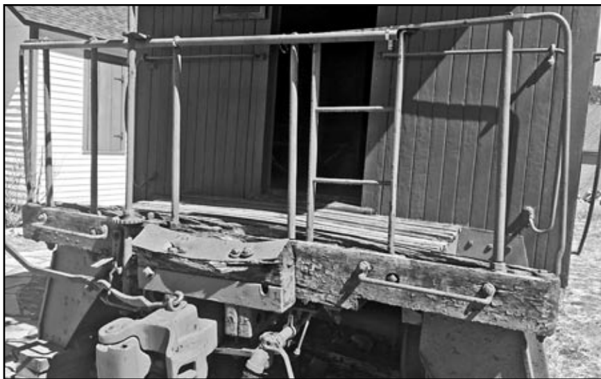
The deteriorated end sill on caboose 10600. – Photo © 2018 Pat Mauro.
