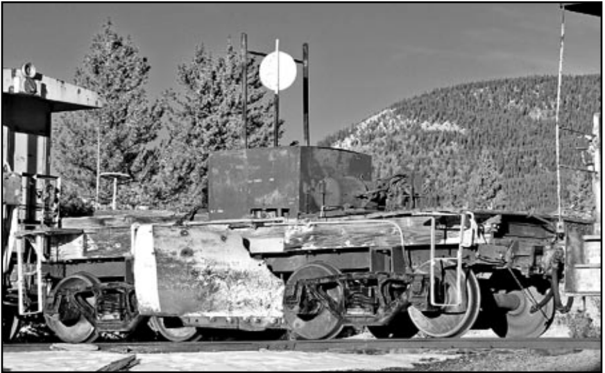
The Leadville flanger was built at Burnham in December 1909 as D&RG #063 and rebuilt with a steel frame in 1941. The Rio Grande sold it to the Colorado & Southern in 1975 and the Leadville, Colorado & Southern Railroad, the current owner, got it when it acquired the C&S Climax branch. It is shown here at Leadville, Colorado, on November 29, 2011.
