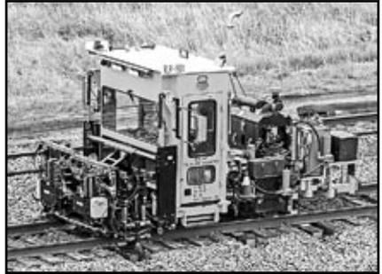
It is followed by the tie plate machine which slightly lifts the rails to position the tie plates so its shoulder hits the outside of the rail.
