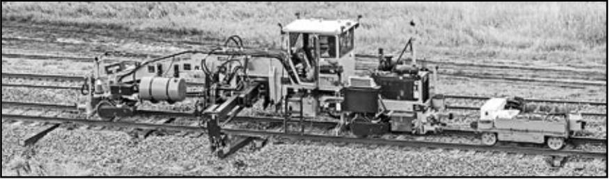
Two long machines follow to slightly lift the rail and properly insert the tie the rest of the way. – Four Photos this page © 2017 Linda Fike.
