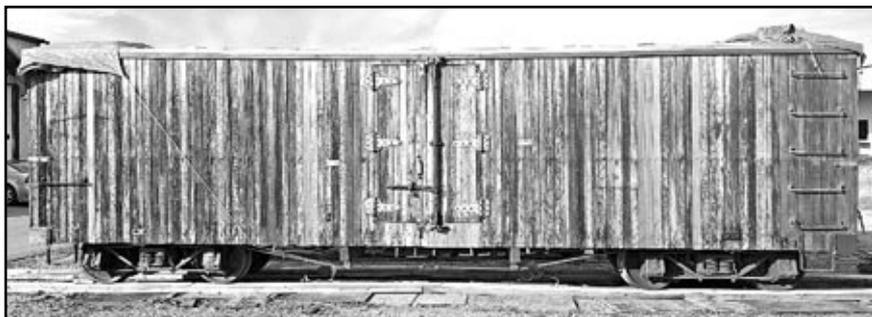
On November 10, 2017, D&RGW Reefer 39 is on trucks again – for the first time in 60 years! Only a few sheathing boards were replaced on the side shown above, since it was protected by being inside the building of which it was a part for about 57 years. The opposite side, exposed to weather, had many boards replaced.
